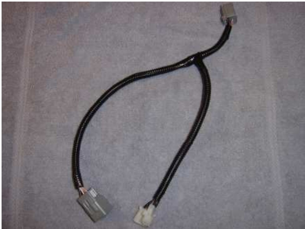
3-Tape through the split in the loom, then wrapped around loom
