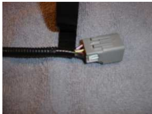
3-Tape through the split in the loom, then wrapped around loom
